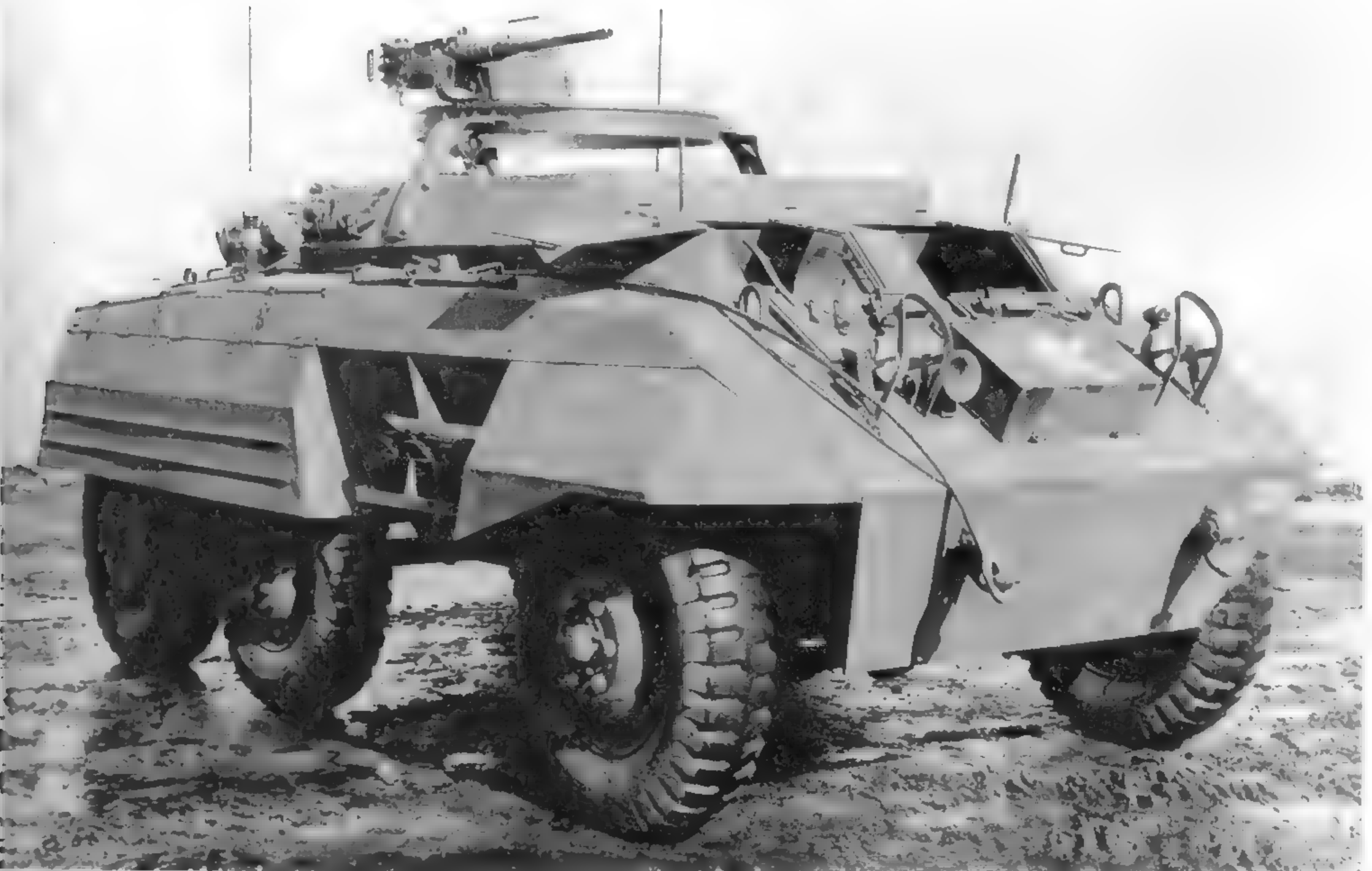
Two-piece hatches were provided for the driver and assistant driver on both the M8 and the M20. The tow cable can be seen here. The M20 had its machine gun mounted on a ring mount. (U.S. Army photo)
